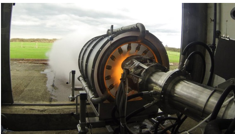
STOIC engine firing with water sound suppression
