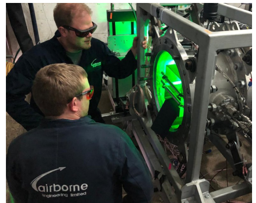
Laser instrumentation on a combustion test rig
