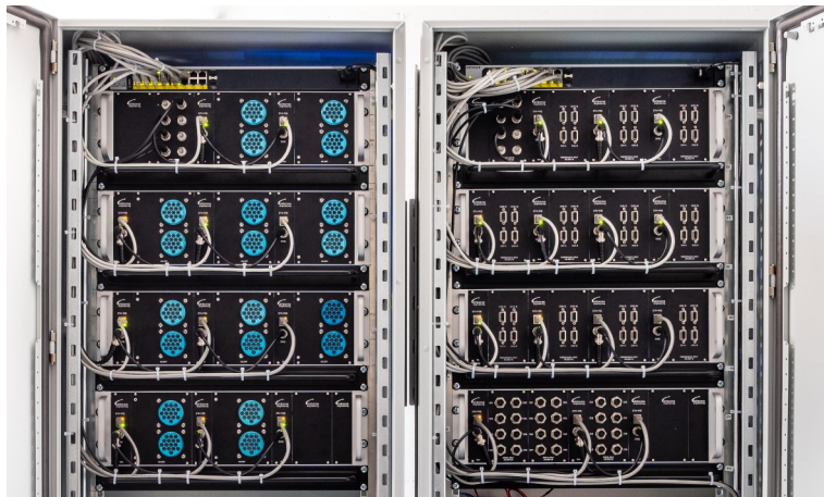
Instrumentation cabinets with 360 channels at 10kHz sample rate
