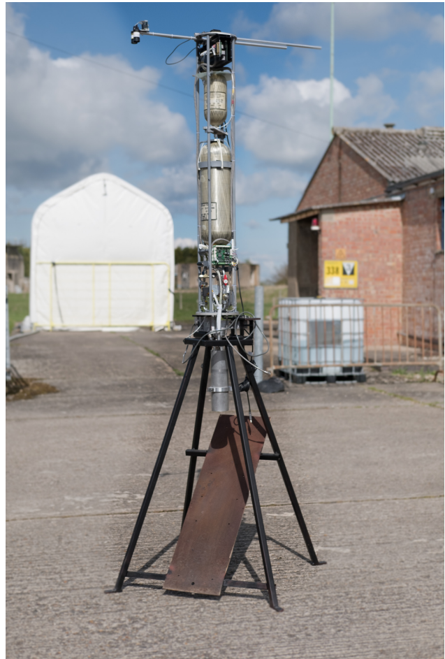
Figure 5: Gyroc vehicle as built, configured for static-tests mounted on a heavy thrust measuring structure
