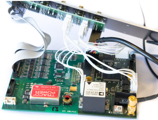
Figure 4: Main GNC avionics board, designed by AEL, featuring a 10-DOF IMU, GPS and interface to external LIDAR.
