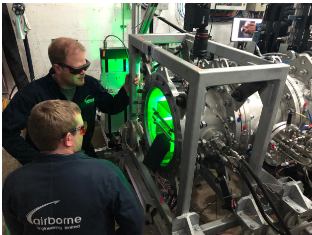
Figure 7: Reaction Engines' Preburner injector test rig for evaluating the combustion performance of the injectors for the SABRE engine preburner.
