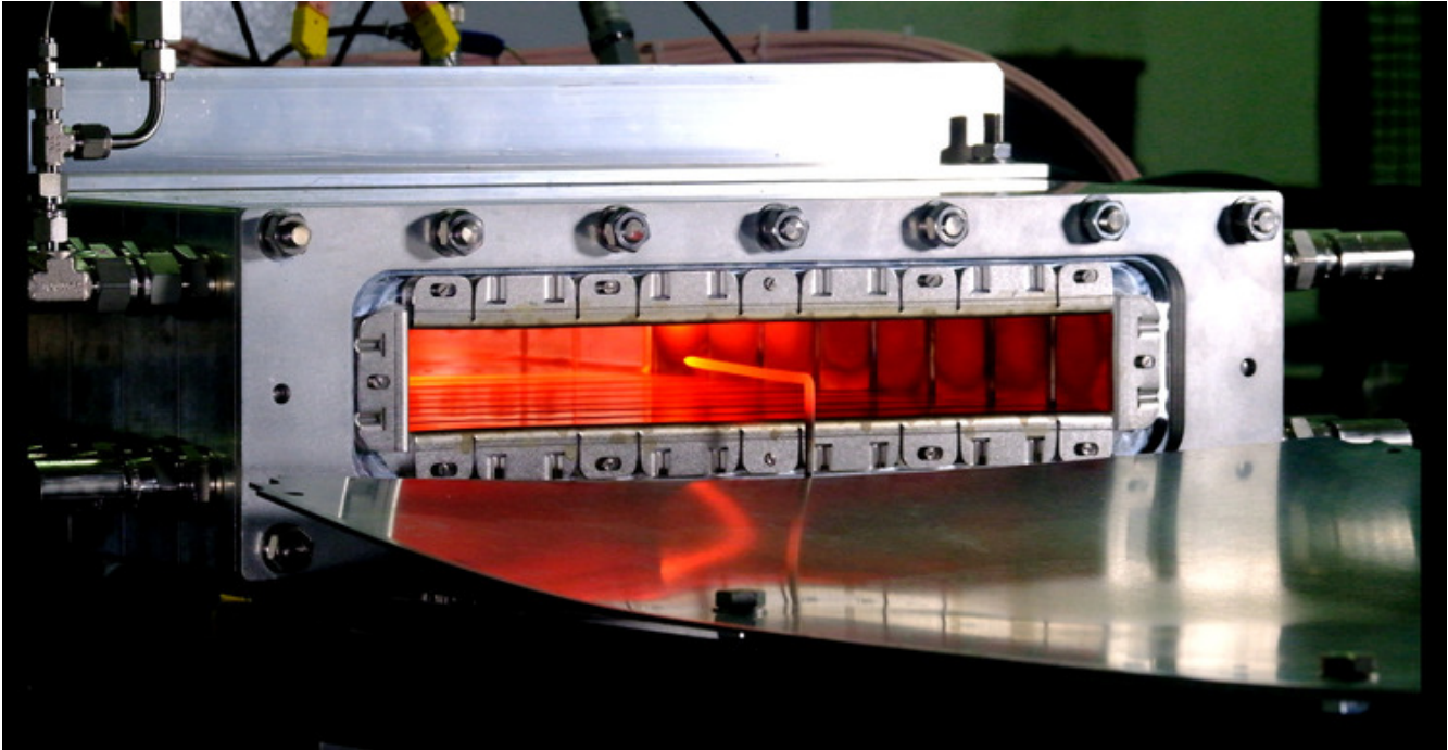
Figure 5: Testing of the vitiated air hot-gas source for testing a single module of the HX3 subsystem for customer Reaction Engines' SABRE engine. A pitot probe on a traverse is used to check flow uniformity in temperature and velocity.
