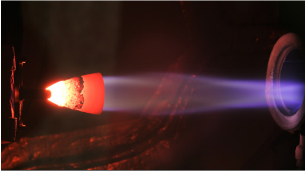
Figure 11: LEROS 10 undergoing a steady-state firing test at the Nammo F-Site High Altitude Facility.
